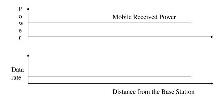
In a Classical Spread Spectrum, the base station controls the power to maintain a constant data rate & Quality of service
