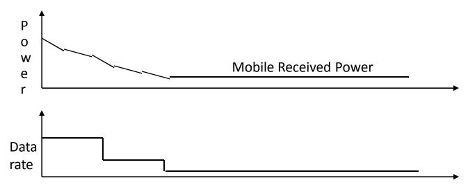
In an 1x EV-DO system, the base station controls the rate of data transmission given a constant transmit power
